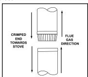
Figure 11A - Chimney Connector
